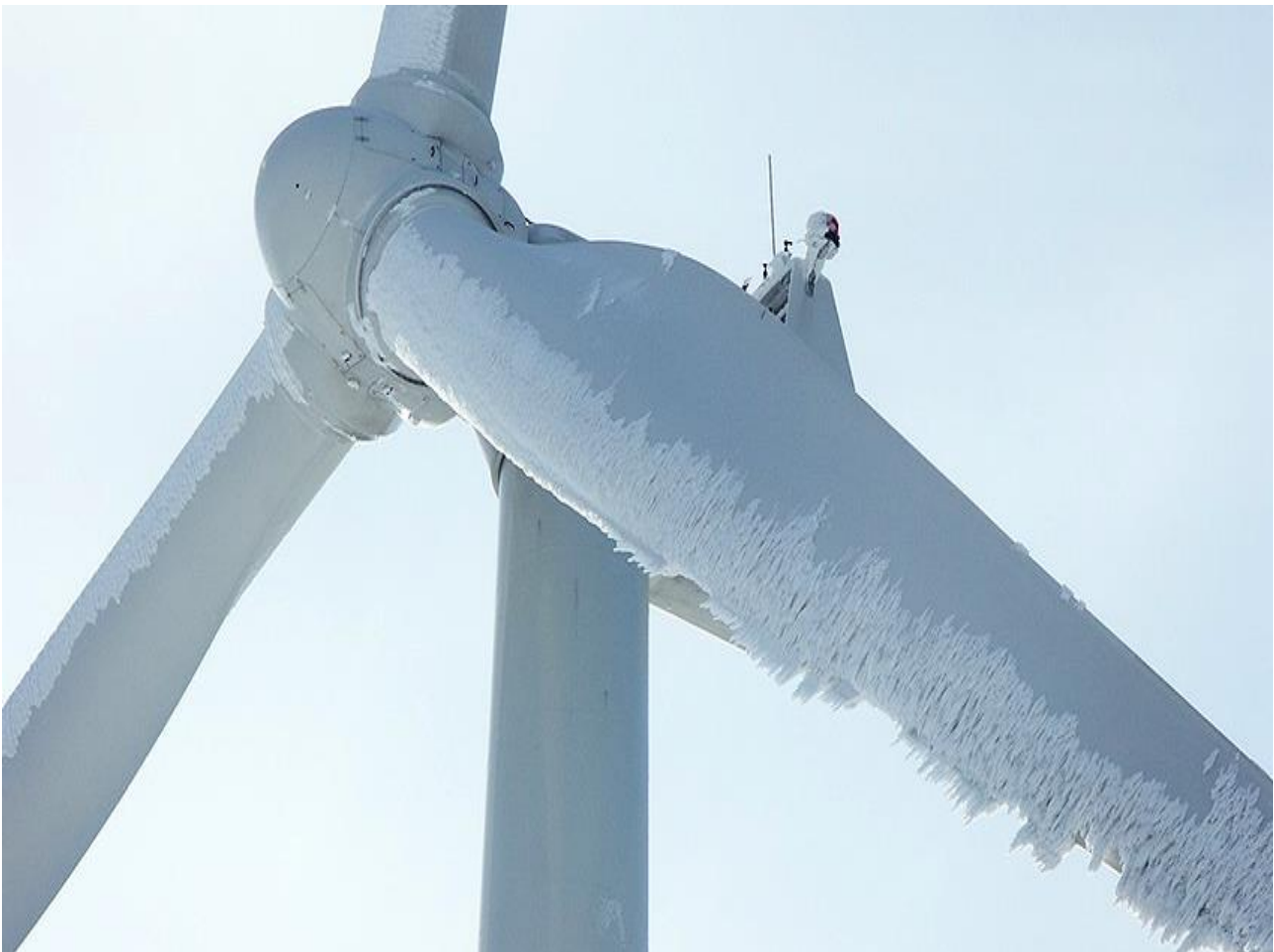
Fig. 1. Example of icing on a wind turbine blade
