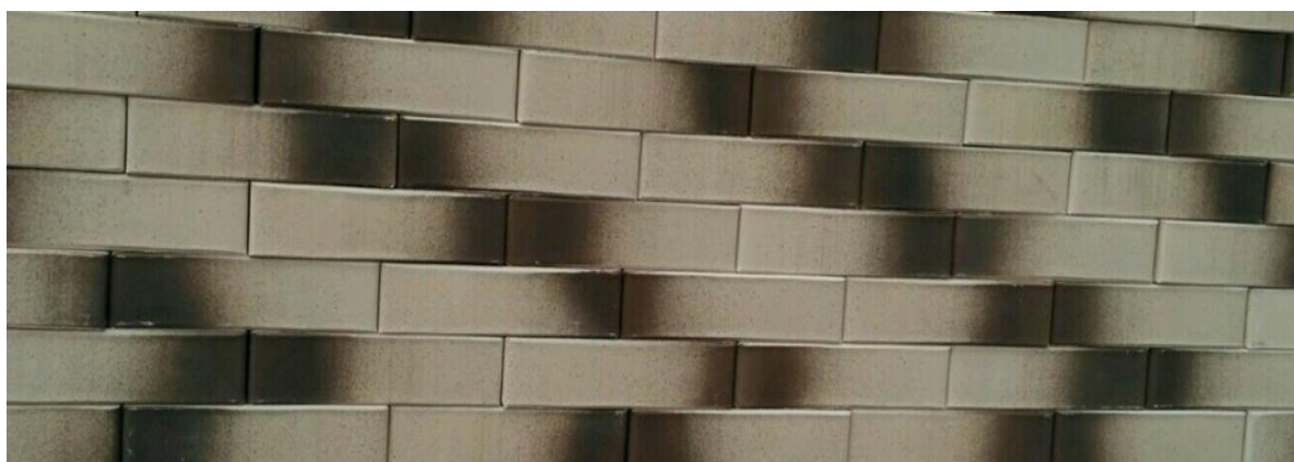
Fig. 10. Decorative bricklaying (engobe compositions B-2, K-4 and G-1)
