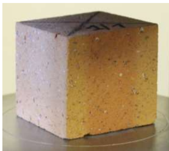
Fig. 7. Ceramic bricks in the section: different color of the outer and inner layers
