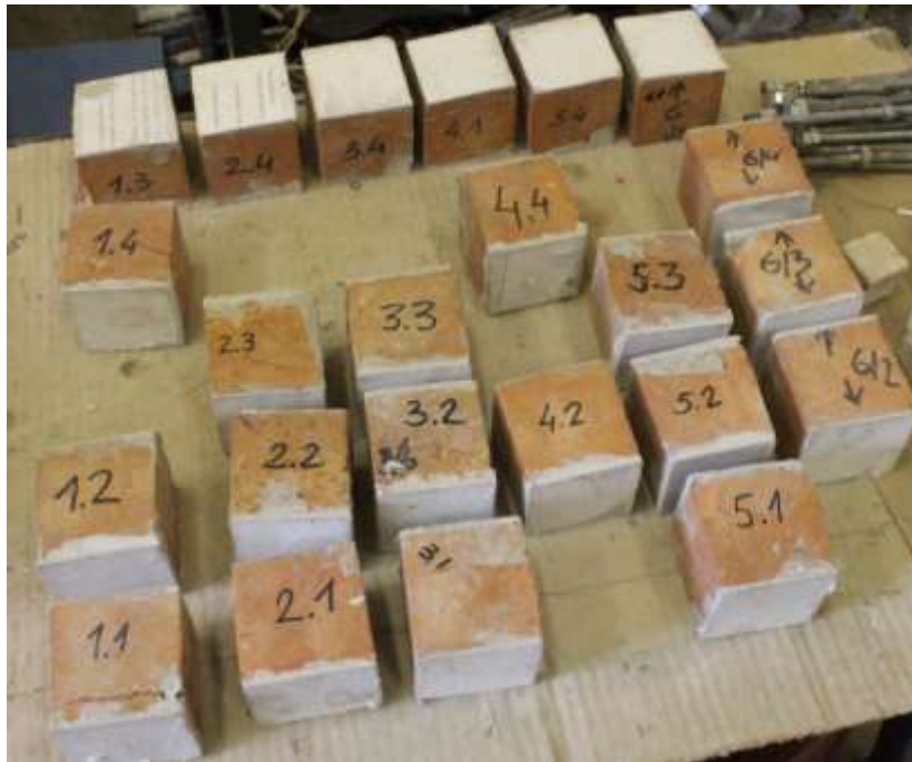
Fig. 3. Ceramic cube samples prepared for the tests
