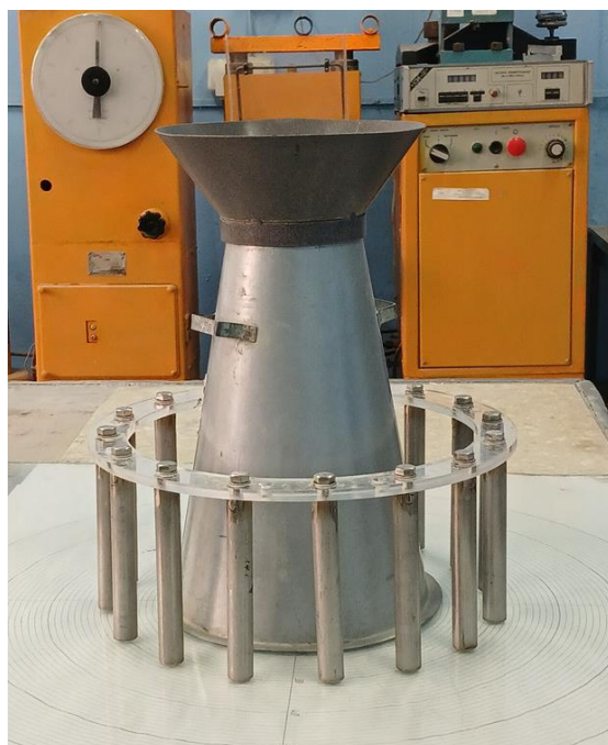
Fig. 1. Device for identifying the self-compaction and fluidity of the concrete mixtures
