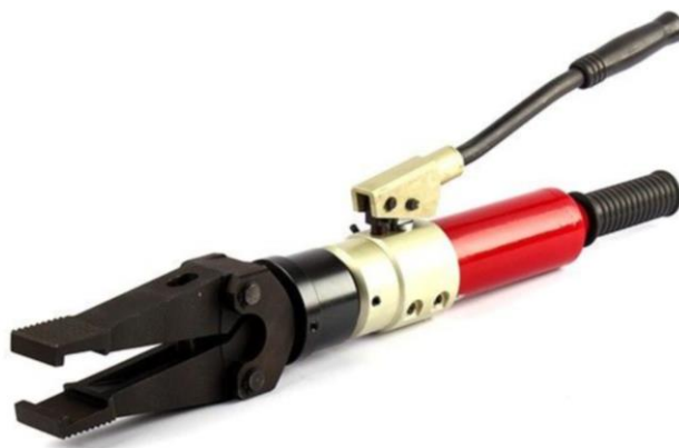
Fig. 5. General view of the self-contained release wedge of the KRA1150 brand
