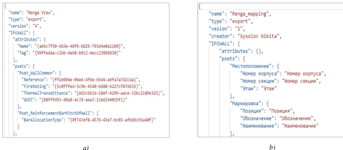
Fig. 6. File for mapping export parameters to IFC for Renga Professional: a — standard mapping file; b — matching file based on the expert evaluation requirements
