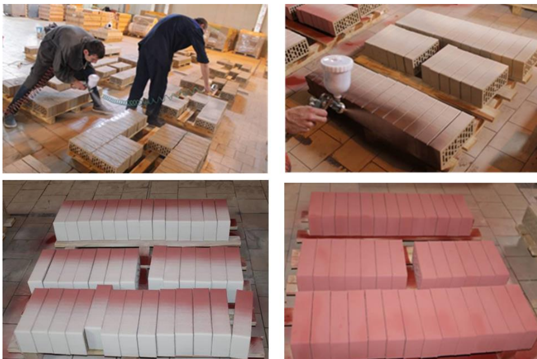
Fig. 4. Engobing by means of airbrushing in the factory setting
