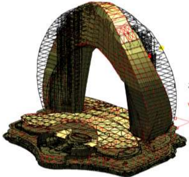
Fig. 12. Second form of own oscillations, f_2 = 0.459 Hz [15]
