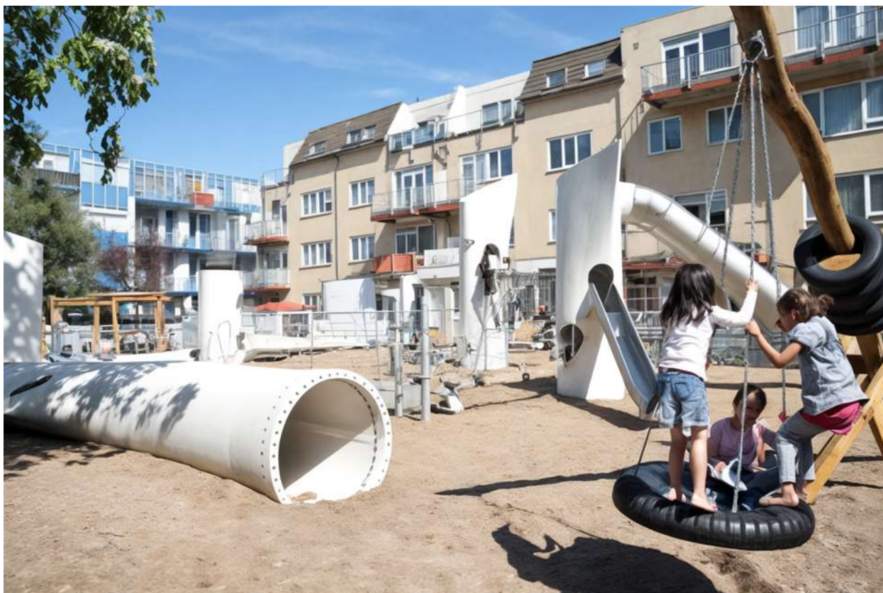
Fig. 1. Architectural solutions for a playground in Rotterdam designed by means of WT blades
